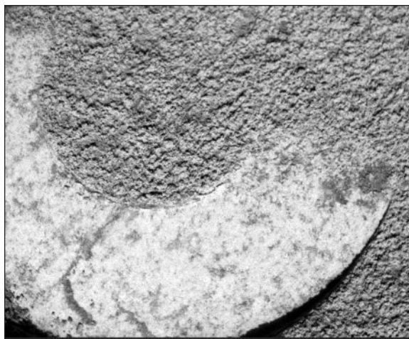
Fig. 1. MI image of soil target at Sugar Loaf Flats, showing partial annular imprint of Mössbauer contact plate. Contact plate was not parallel to soil surface, so contact was made only in the brighter part of the image. The part of MI full frame 2M1321-32632 shown here is 27 by 22 mm. Illumination from bottom.
